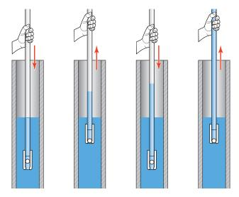
Inertial Pump Operation
