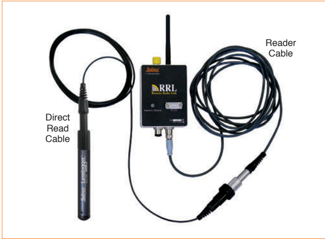
Levellogger Connection to the RRL Station
